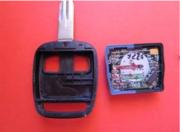
2. Next prise open your remote end up with 2 parts: One consisting of hard shell with battery, second part being top part of the shell with electronic board button keypad.
