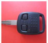
6. Close shell by placing bottom part of the shell with battery over top part consisting of keypad and electronic board.
